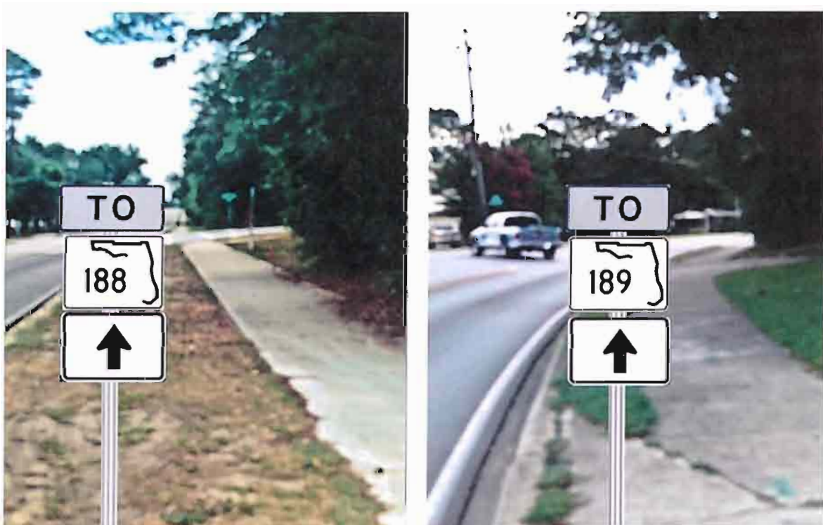
Figure 6. Recommended State Route Signs on Mooney Road
